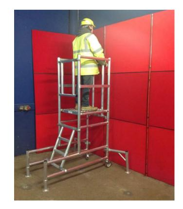
Dimensions — Platform at 1.25M x Width –0.65M x Depth 1.3M Working Height— 3.25M (Max) Dimensions — Folded Height –2.26M x Width - 0.25M x Depth - 1.3M Weight— 33Kg Safe Working Load - 150kg PAS 250— 36Kg(Mini Stabilisers) PAS 250— 39Kg(Std Stabiliisers ) Manufactured under an ISO9001:2008 Quality System Complies fully with the Working at Height Regulations 2005 and PAS250 Specifications Lightweight all Aluminium Construction
